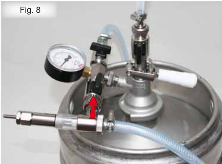
Open ball valve II (CO<sub>2</sub> line). CO<sub>2</sub> vents until non-return valve closes. Keg is now full.
