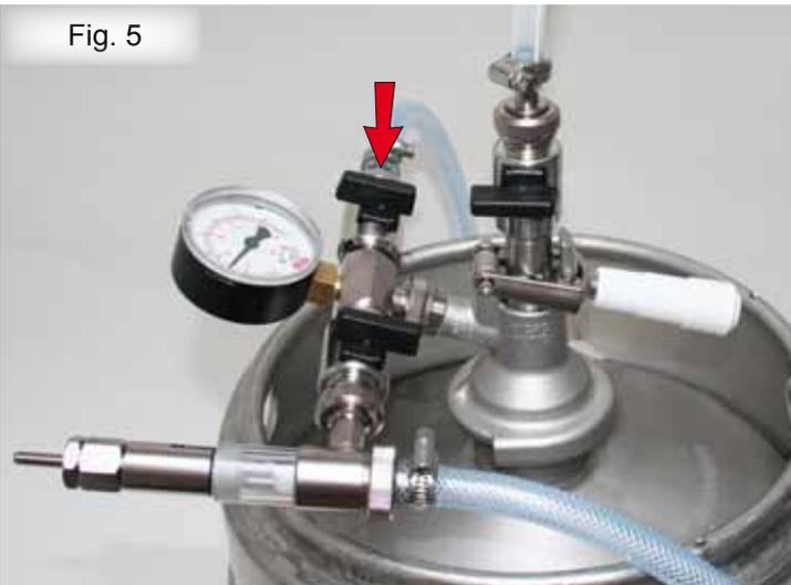
When the correct pressure (about 1 bar) shows on pressure gauge close ball valve I.
